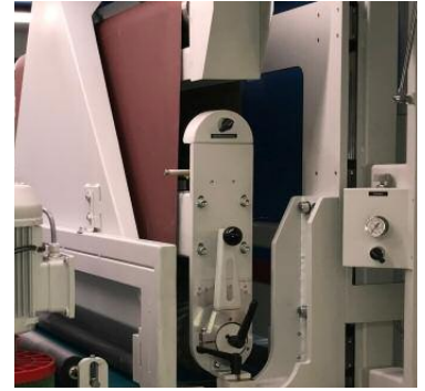
Abrasive belt unit with floating head system
